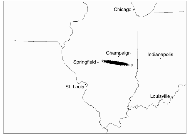
Fig. 13 Range dispersion at atmospheric interface resulting from over 3500 Monte Carlo simulation cases.
